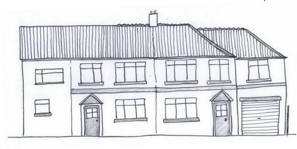
Figure 7 Two storey side extensions
